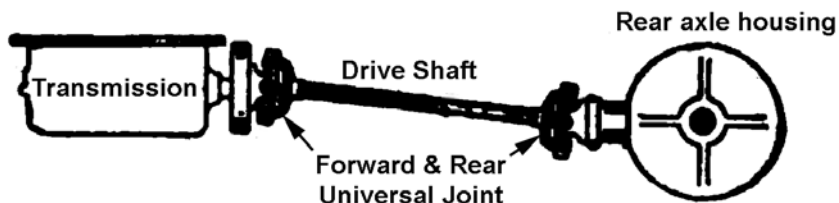
SCHEMATIC SECTION OF UNIVERSAL JOINT CONNECTIONS BETWEEN TRANSMISSION AND REAR AXLE
