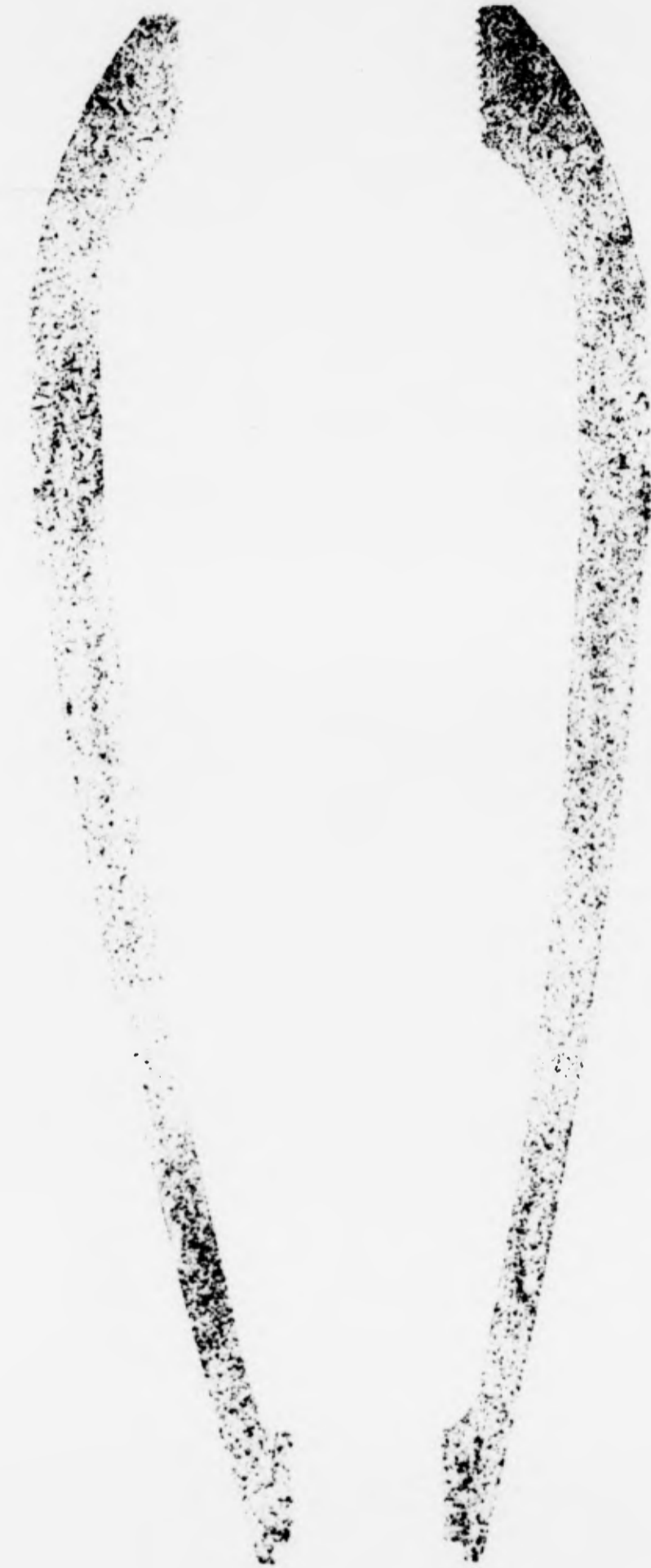
24805 Figure 5. Sulphur Print of Shell No. 111. Actual Size
