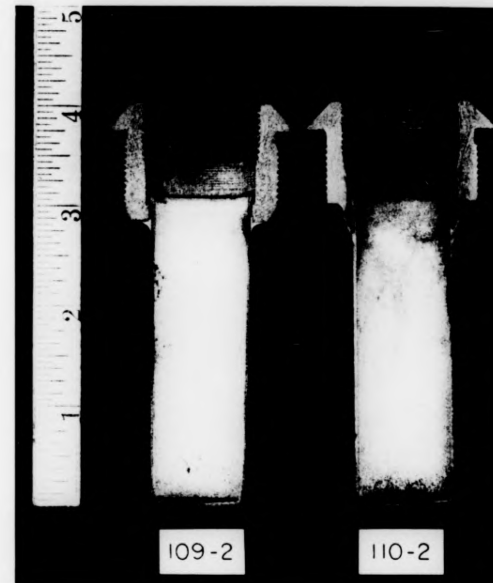
25031 Figure 6. Deep-Etched Sections of Two Booster Cups and Adaptors.
