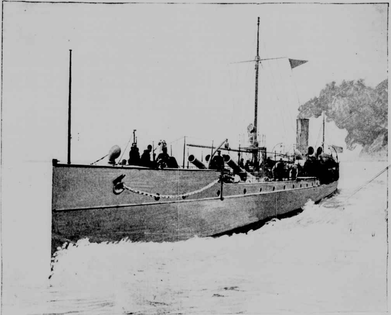
DYNAMITE GUN VESUVIUS. 300 tons; 1,734 horse-power; 23 knots speed. Lieutenant-Commander John R. Pillsbury commanding.
