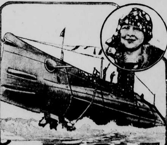
Above are shown the S-47, the last word in undersea fighting craft, as she left the ways of the Electric Boat company's Fore river plant at Quincy, Mass., and Mrs. Morris D. Gilmore, wife of Commander Gilmore, who used spring water in christening it. This new United States submarine has a cruising radius of 8,000 miles at one filling, a surface speed of 14 knots and a submerged speed of 12 knots.
