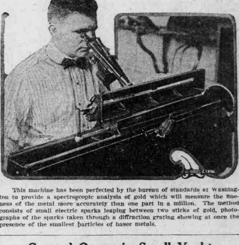
This machine has been perfected by the bureau of standards at Washington to provide a spectroscopic analysis of gold which will measure the fineness of the metal more accurately than one part in a million. The method consists of small electric sparks leaping between two sticks of gold, photographs of the sparks taken through a diffraction grating showing at once the presence of the smallest particles of baser metals.
